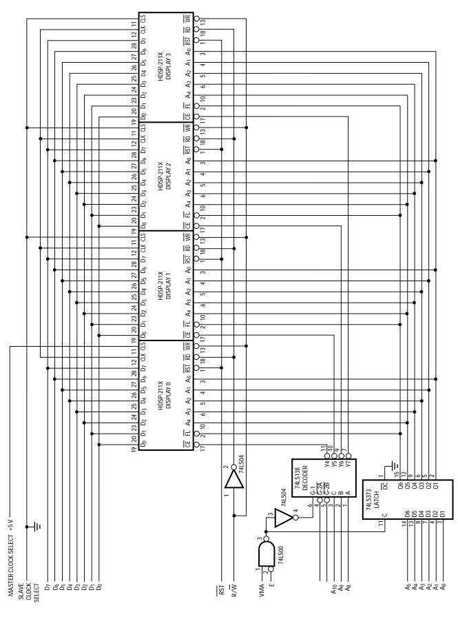
Figure 1. 32 Character Interface to 6808 Microprocessor
