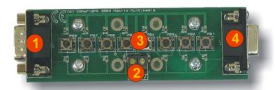
This simple switch panel contains 8 push-to-make switches – one for each line on the E-blocks port.
