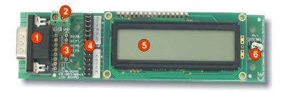
This 2 line 16 character alphanumeric LCD display uses 5 lines of the E-blocks to allow the display of numbers and characters on the display
